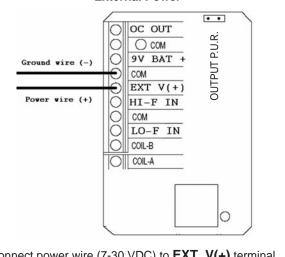
Connect power wire (7-30 VDC) to **EXT\_V(+)** terminal. Connect ground wire to any **COM** terminal.
